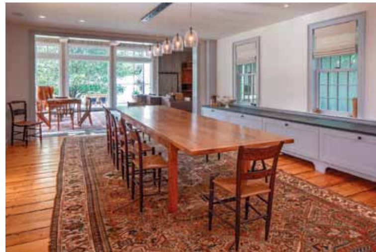
Shifty sideboard. To disguise the sag of the 230-year-old floor—nearly 3 in. out of level in a span of 15 ft.—the builder made a base with different-length legs. The gap between the bottom rail and floor varies along the length of the piece, but because the shadowline masks the incremental height differences, the eye doesn't pick up on it.
