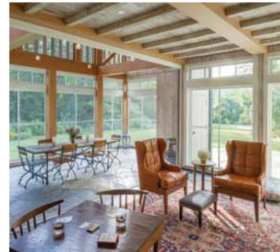
Rustic respite. LVLs wrapped in chestnut warm the partially conditioned interiors, which are separated from the screened porch by a NanaWall that disappears from view when open.
